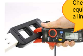
Measuring current of small devices in tight spaces
