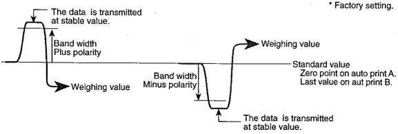
Case of plus polarity HP/HF/HM/HR SERIES
