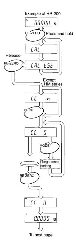
Place the target mass on the pan and press the RE-ZERO key. The balance weighs the mass value and outputs the "Calibration test report".
