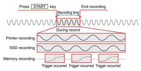
When the START key on the operation panel is pressed, recording to the various devices specified in the [Setup] menu starts, and continues until the time set in [Recording time] in the recording setup elapses or the STOP key on the operation panel is pressed. Memory recording records the input data to memory when the trigger is occurred after recording starts. Data recording is not performed unless a trigger is detected.
