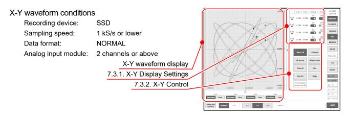
By tapping the **[**Single/Quad**]** key for display control, the X-Y waveform can be displayed as four waveforms overlaid on a single screen or as four separate screens.
