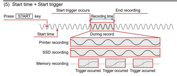
When the <u>START</u> key on the operation panel is pressed, this product enters the measurement standby state after the time set in [Start time]. Recording to the various devices starts when the channel trigger specified in [Start trigger] is occurred, and continues until the time set in [Recording time] in the recording setup elapses or the <u>STOP</u> key on the operation panel is pressed.
