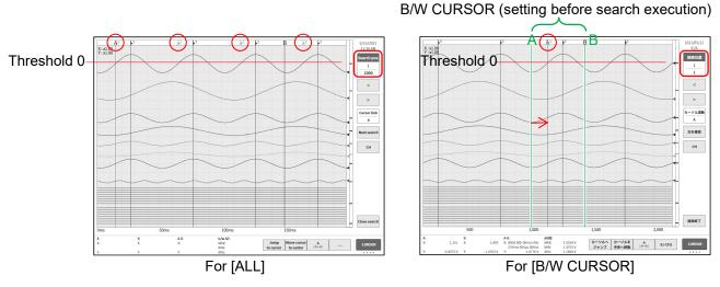
The figure above is the search result when the search setting is LEVEL UP and the threshold is set to 0. The search is executed for the topmost sine wave (1,000 waves or more).
