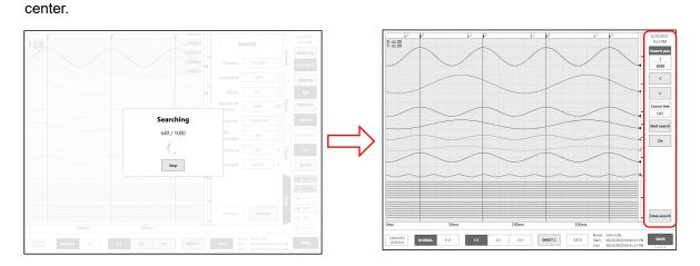
Step 6. When there are one or more search results, press the [<] key (back)/[>] key (forward) in the "7.5.10. Search Display Menu" to change the waveform display. You can press the [CH] key to return to the channel setup sub menu and reset the search conditions. Press the [Close search] key to return from the "7.5.10. Search Display Menu" to the basic side menu.
