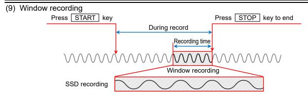
When the START key on the operation panel is pressed, recording to the various devices starts, and continues until the STOP key on the operation panel is pressed. The data of the time set in [Recording time] until stop is recorded to the SSD.
