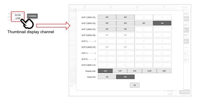
Display scale: 1/10, 1/20, 1/50, 1/100, 1/All Making the scale smaller (with a larger decimation number for the data to display) displays a wider time range of the waveform, because the number of points to display is the same. 1/10 is the 10 x time range, and 1/50 is the 50 x time range.
