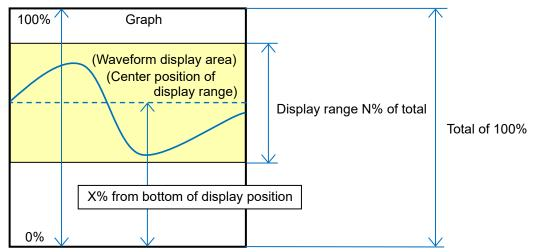
Description of Step 6 (setting the display maximum and display minimum (waveform display scale))
