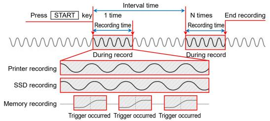
When the START key on the operation panel is pressed, recording to the various devices starts and continues until the time set in [Recording time] in the recording setup elapses, and then the next recording starts when the time in [Interval time] elapses after measurement starts. Measurement ends when recording has been performed the number of times specified in [Number of Recording times] for the interval.
