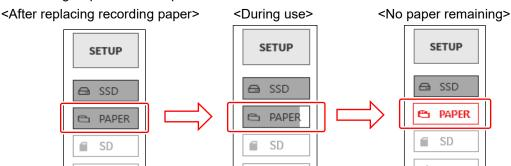
Reset the remaining paper monitor after replacing the recording paper. Press and hold [PAPER] (remaining paper monitor) on the side menu to display the dialog box for resetting.
