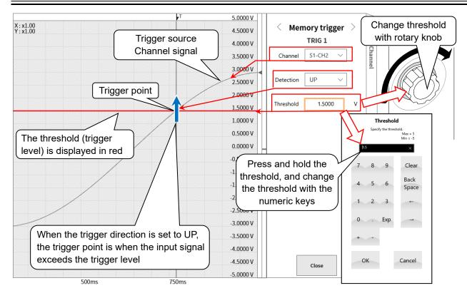
Description of trigger source (3) Detection and (4) Threshold
