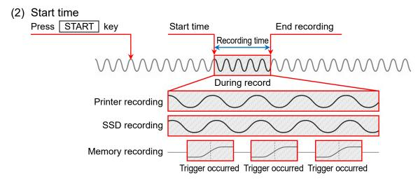
When the <u>START</u> key on the operation panel is pressed, this product enters the measurement standby state and recording to the various devices starts at the [Start time] set in the recording setup, and continues until the time set in [Recording time] in the recording setup elapses or the <u>STOP</u> key on the operation panel is pressed.
