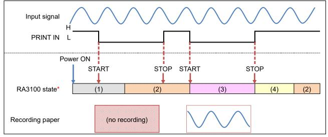
\* The states of the RA3100 are (1) Starting up, (2) Measuring, (3) Printing, and (4) Stopping printing.
