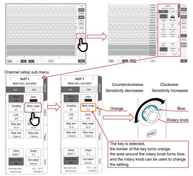
Step 5. Tap the [CHx] tab in the channel setup sub menu to change the displayed channel.
