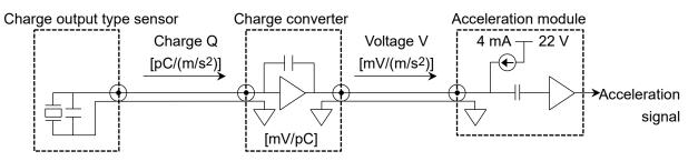
A charge output type acceleration sensor is lightweight and compact, and is suitable for measurement at low or high temperatures.
