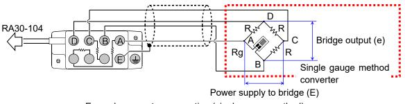
Example converter connection (single gauge method)
