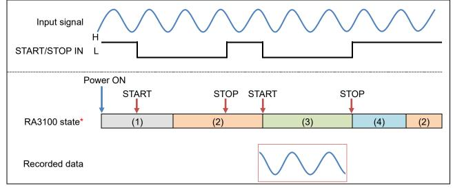
\* The states of the RA3100 are (1) Starting up, (2) Measuring, (3) Recording, and (4) Saving recording.
