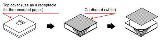
Step 2-2. Place the paper in the stock box with the thermally sensitive side (the side with blue numbers printed on the edges) facing up.
