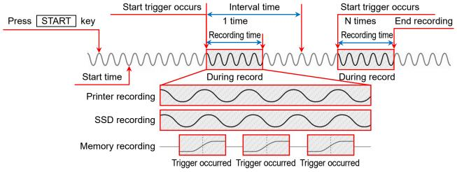
When the START key on the operation panel is pressed, this product enters the measurement standby state and starts the procedure indicated in "(6) Start trigger + Interval (N times)" at the time set in [Start time].
