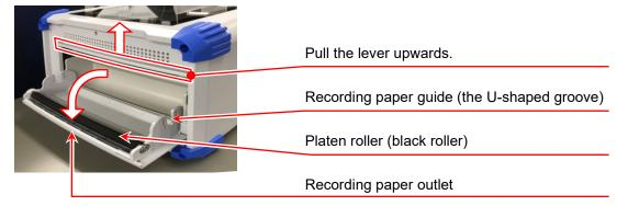
Step 3. Load the paper following the guide of this product, and press the paper holders into the guide until a click is heard.
