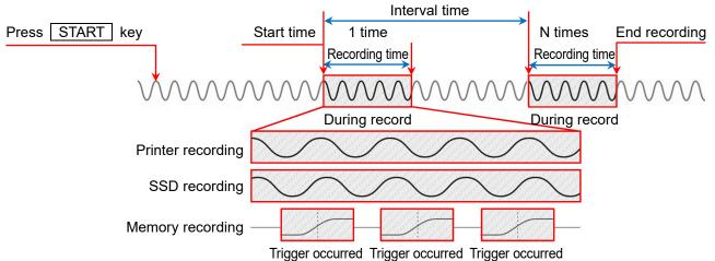
When the START key on the operation panel is pressed, this product enters the measurement standby state. Recording starts at the time set in [Start time], then continues recording for the time set in [Recording time].
