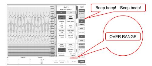
Step 3. Set the input filter. Set the low-pass filter with the [L.P.F.] key (8).
