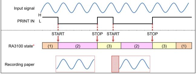
\* The states of the RA3100 are (1) Measuring, (2) Printing, and (3) Stopping printing.
