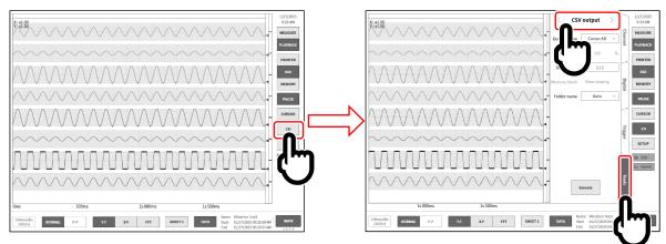
Step 6. Select the conditions for outputting the CSV file in [CSV output].
