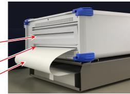
Step 4. Thread the paper through the Z-fold paper adapter. Thread the paper inserted into the opening under the printer cover through the Z-fold paper adapter as shown in the figure.
