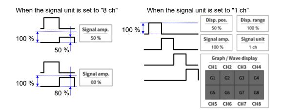
(11) Signal unit: Sets whether to assign channels to the graph on a single channel basis or eight channel basis.
