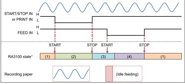
\* The states of the RA3100 are (1) Measuring, (2) Recording or printing, (3) Saving recording or stopping printing, or (4) Feeding.
