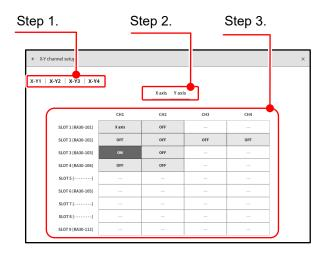
Step 4. When the settings are complete, tap  $[\leftarrow]$  or [x] on the top title bar to return to the original X-Y waveform display.
