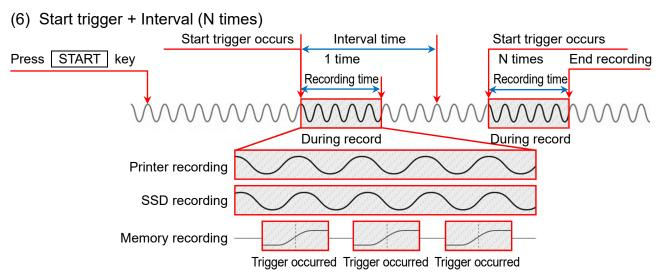
When the <u>START</u> key on the operation panel is pressed, this product enters the measurement standby state and recording starts when the channel trigger specified in [Start trigger] is occurred. Measurement continues until the time set in [Recording time] in the recording starts elapses, and then the next recording starts when the time in [Interval time] elapses after recording starts, and this product waits for the next start trigger.
