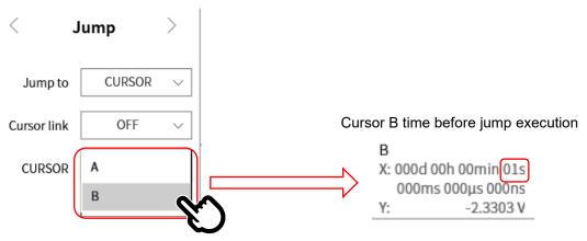
Cursor B (time 1 s) is displayed in the center of the Y-T waveform.
