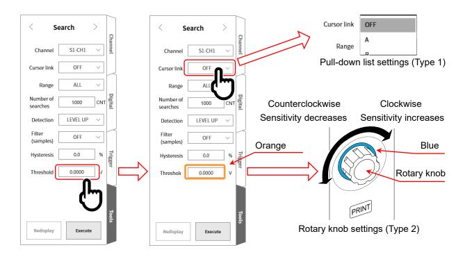
Step 5. When the settings are complete, tap the [Execute] key. The search starts, and when the search is complete, the S mark and the waveform near the results are displayed on the Y-T waveform, and the side menu switches to the "7.5.10. Search Display Menu." The display position of the S mark changes according to the display position of the search results.
