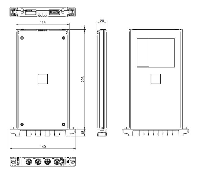
12.4.4. 2ch High Speed Voltage Module (RA30-103) Exterior
