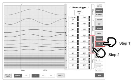
Step 3. Up to 18 trigger sources (【T1】 to 【T18】) can be set.Tap the number of the trigger source to set to display the details screen.
