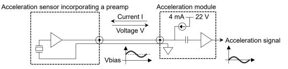
An acceleration sensor incorporating a preamp is a sensor where the charge output type acceleration sensor and preamp (charge converter) are integrated.
