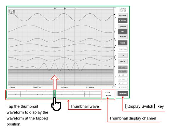
The thumbnail waveform displays the display area of the Y-T waveform and the positions of Cursor A and Cursor B.
