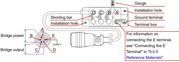
Example bridge box connection (single gauge method)
