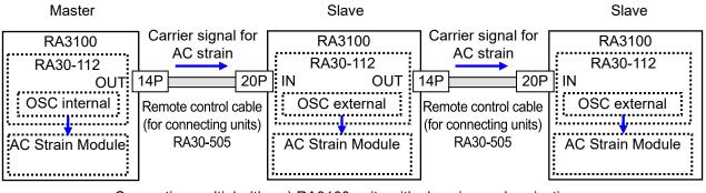
Connecting multiple (three) RA3100 units with chassis synchronization
