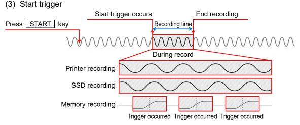
When the <u>START</u> key on the operation panel is pressed, this product enters the measurement standby state. Recording to the various devices starts when the channel trigger specified in [Start trigger] is occurred and continues until the time set in [Recording time] in the recording setup elapses or the <u>STOP</u> key on the operation panel is pressed.
