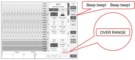
Step 3. Set the input filter. Set the low-pass filter with the [L.P.F.] key (8).
