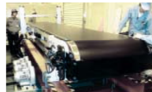
Moving belt under the body of the vehicle
